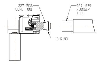
10. INSERT CONE TOOL NO. 227-1538 INTO THE INTERFACE AND SLIDE THE O-RING OVER THE END OF THE CONE TOOL. USING THE PLUNGER TOOL NO. 227-1539, SLIDE THE O-RING DOWN THE THE CONE TOOL AND OVER THE END OF THE BODY. THE O-RING WILL SNAP INTO THE GROOVE AT THE BOTTOM OF THE INTERFACE.
