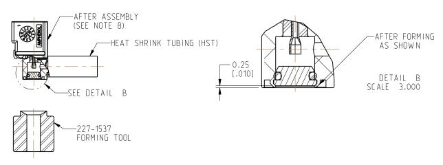
6. INSERT CAP & O-RING INTO BODY AND SWAGE BODY USING TOOL 227-1537.
