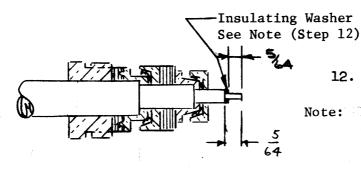
12. Trim inner conductor to dim. shown.
