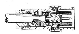
14. Insert completed cable hardware assy. into either Jack or Plug body. Make sure part (2) is properly seated on sharp edge of part (3). After nut is started, Sighten with torque wrench to 13 to 15 in. lbs.
