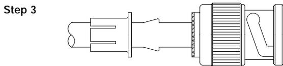
**Step 3** Slide body over contact and cable insulation with barb going UNDER flared braid. Push body until shoulder is against cable jacket. Braid will flare out against body shoulder.
