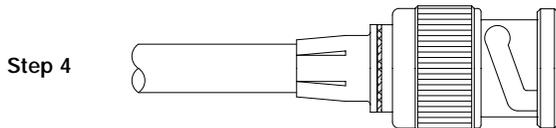
**Step 4** Grasp cable with hand and push ferrule over barb until braid is captured between ferrule and body flange. Assembly is complete.
