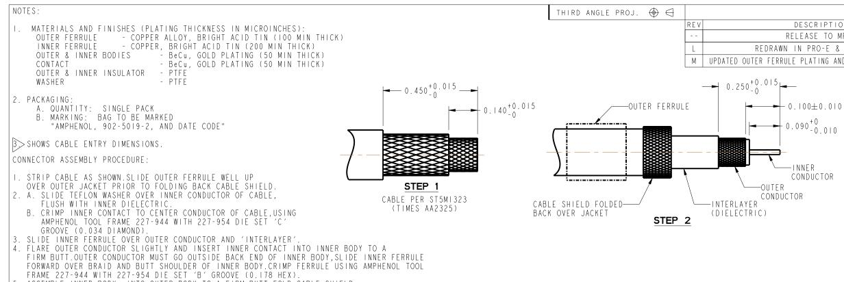
ASSEMBLE INNER BODY INTO OUTER BODY TO A FIRM BUTT, FOLD CABLE SHIELD FORWARD OVER BODY SLIDE OUTER FERRULE FORWARD OVER BRAID AND BUTT SHOULDER OF BODY CRIMP FERRULE USING AMPHENOL TOOL FRAME 227-944 WITH 227-954 DIE SET 'A' GROOVE (0.263 HEX).
