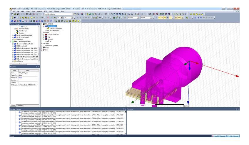
Select the entire component via the side menu and position the component on the launch model so that it is flush with the top of the board. Ensure that no objects are interfering with the component or enable materials override in the HFSS design settings. Note that although the internal geometry is hidden, it will still simulate as normal.
