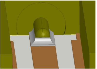
A small amount of solder is already modeled on the center pin, but if an accurate solder model is needed, solder can be modeled on the pad around the center pin as desired. Solder will also need to be modeled around the ground pins of the connector.
