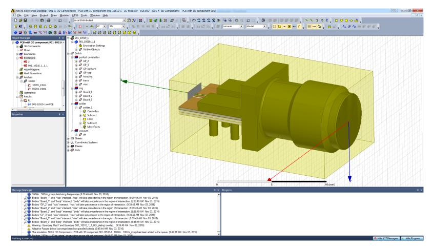
The mated connector interface and input port are already modeled internal to the 3D component. Because of this, the front face of the connector must be against the edge of the airbox. From there, model a board-side port object and analysis setup can be performed as normal.
