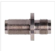
**After 720 Hours of Salt Spray Exposure:**
