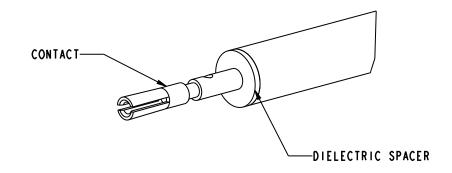
A. INSERT PREPARED CABLE AND CONTACT INTO BODY UNTIL CABLE BOTTOMS INTERNALLY.
